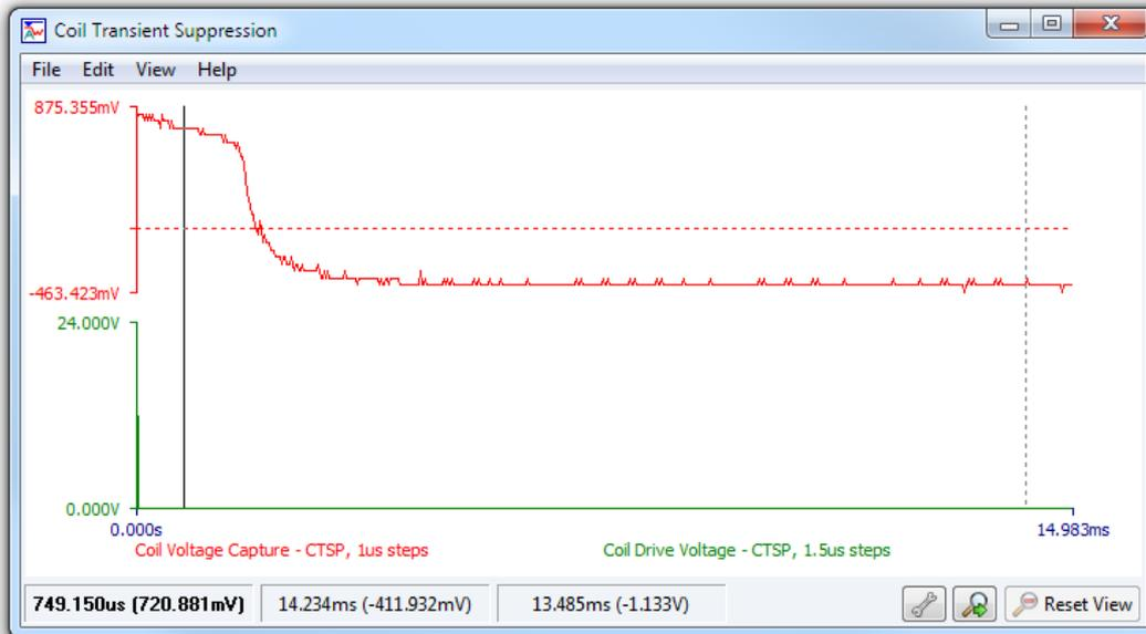
Now the non-zero 'floor' mentioned above can be more clearly seen at around -460mV but the diode clamping action is visible at around 0.875V indicating a correctly functioning diode. It is also usual to see some high-frequency noise appear on the trace due to fixturing and cabling pickup. This can be ignored as long as it is not significant compared to the limit being examined.
