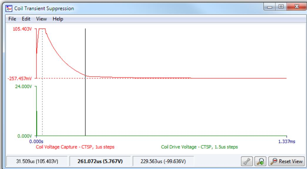
You can see that the lack of coil suppression leads to a large (105V) reverse voltage when the coil is released.
