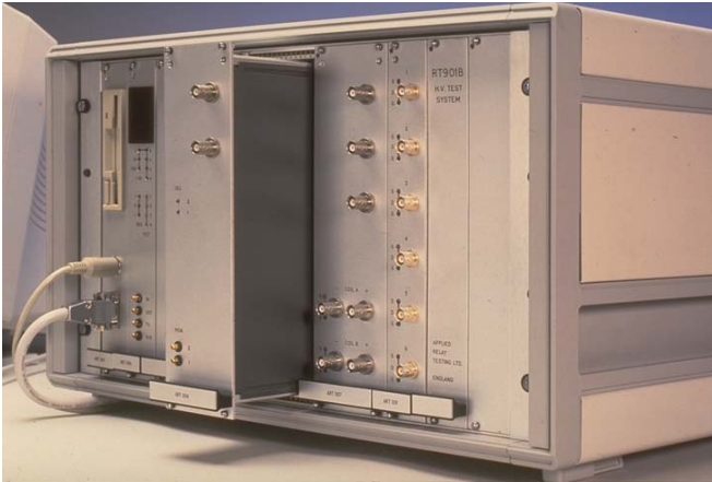
Figure 18. Close-up of an interchangeable high-voltage generator on the RT901.
