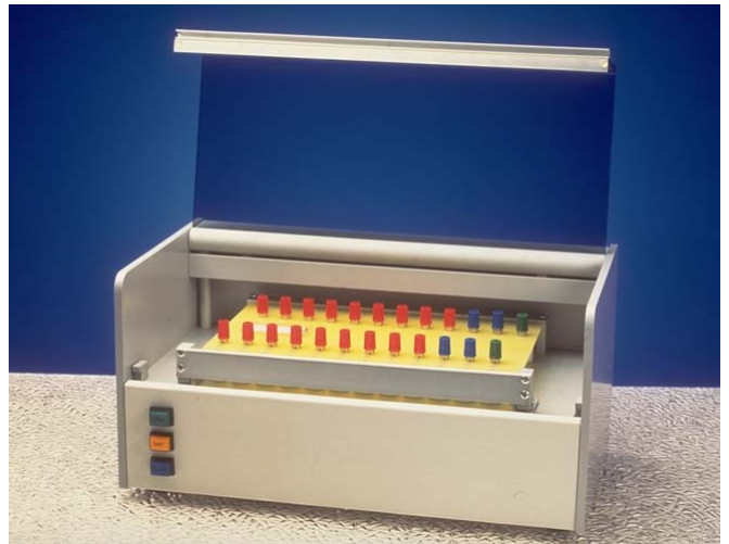
Figure 26. Test fixture with a general-purpose 4mm terminal adaptor installed.
