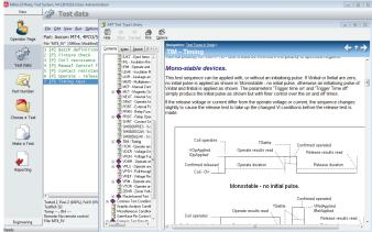
Artworks provides a feature rich user interface for ART's RT290 and full range of Reflex test systems. It integrates customisable spread sheet based test program generation, user interface and report generation all with built-in context sensitive help documentation.
